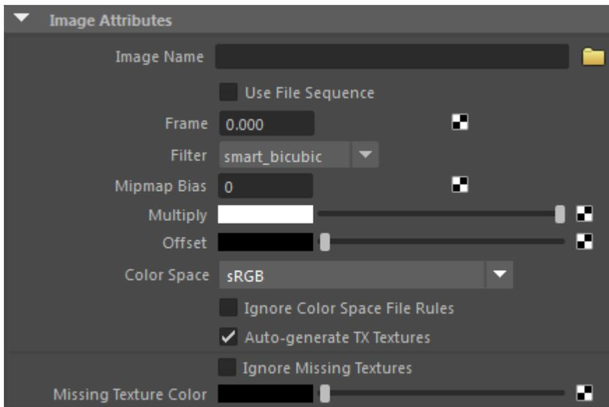
The 'Image' node is a color shader which performs texture mapping using a specified image file. You can control the position, size, and rotation of this frame on the surface. You can control how the texture is tiled within the frame using the Scale UV, Flip, Wrap and Swap attributes.
